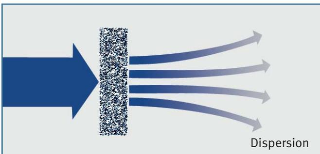
Good dispersion of liquids within the Fibre felt material and high suction effect due to the high porosity. Various applications, e.g. in ink cartridges.
